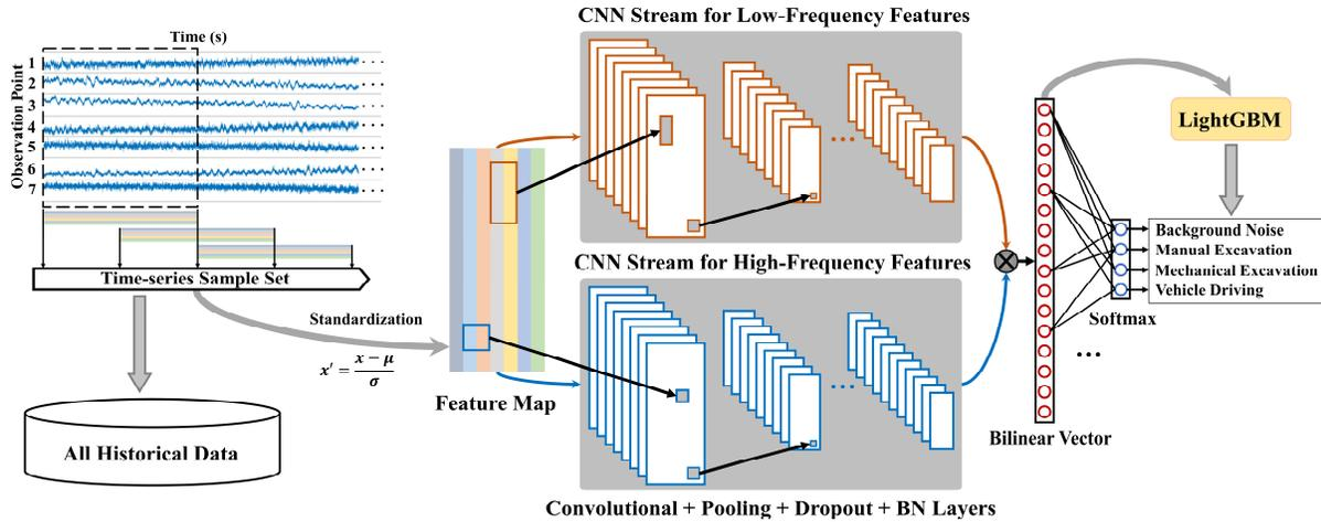
**Fig. 1.** Data pre-processing and structure of the proposed B-CNN and LightGBM model. More specifically, we changed the size of the input and the output matrix to allow our data to be trained, and we adjusted the size and the initial weights of the convolutional kernels and added the pooling and the batch normalization strategies in the two CNN streams of the original B-CNN [18,19], intending to better fit our distributed data.
